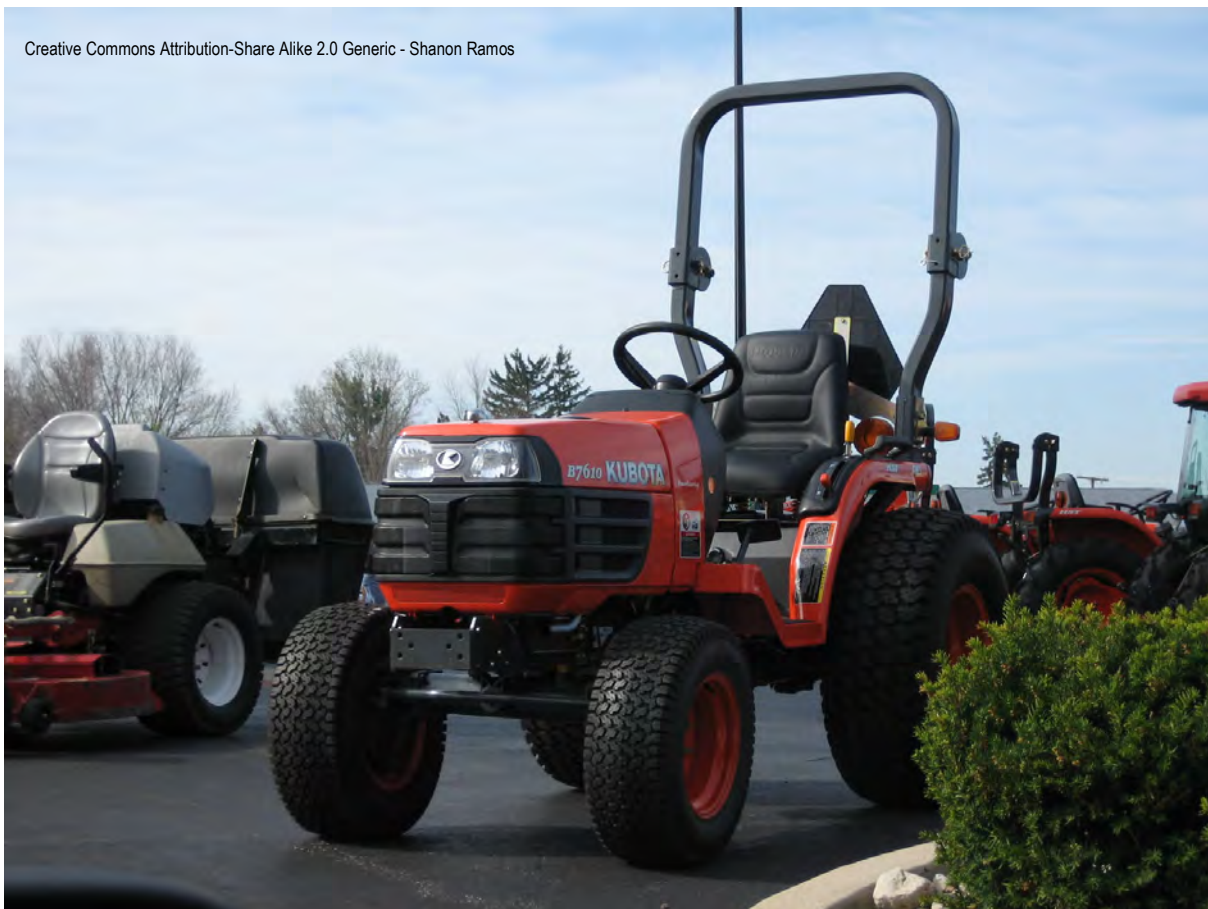
Figure 9: Tractor fitted with a roll-over protection system
